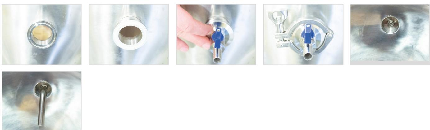
The bottom hole in the fermenter is for mounting the large butterfly valve. You can choose to mount the elbow first. Proceed in the same way as with the above tap.
